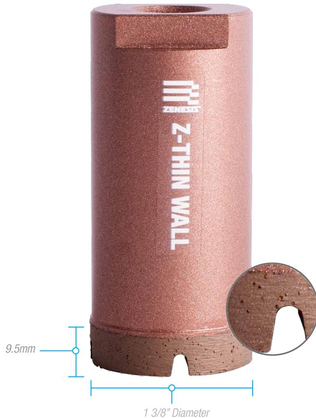
The **ZENESIS™ Z-THIN WALL CORE BIT** makes the cleanest holes in the largest variety of materials. The unique continuous thin rim is extremely precise and fast. They are great for marble, granite, engineered stone, porcelain and sintered stone. This bit has far less chipping on the top and less blow out on the bottom when compared to standard core bits.
