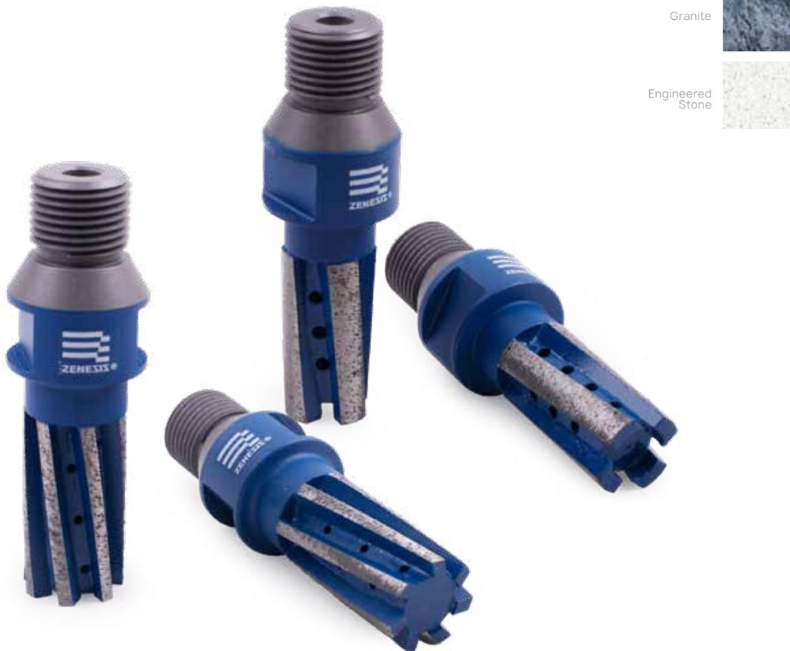
The all-new **ZENESIS™ 4 AND 7 SEGMENT FINGER BITS** provide top CNC performance on all stone materials. They deliver precise, quiet and chip-free cutting at faster speeds and can be used on soft to medium-hard materials (4 segments) or medium to hard materials (7 segments). The enhanced design utilizes our most advanced diamond pattern to date, which increases durability and prevents premature wear to ensure long tool life.
