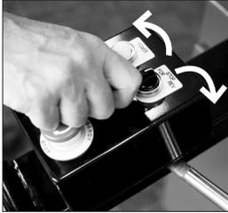
4. Use the Direction Control Switch to set up the direction of rotation.
