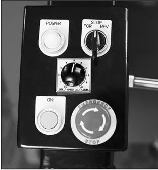
The 'ON' Button, when pressed, turns the power on when the Emergency Stop button has not been engaged. Check that the Emergency Stop button has not been engaged by turning it clockwise.
