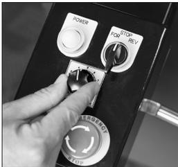
6. With grinding heads on the working surface, push the "On" button to start the machine, push down on the handle just enough to release the pressure off the diamonds, but don't lift machine completely off the floor.
