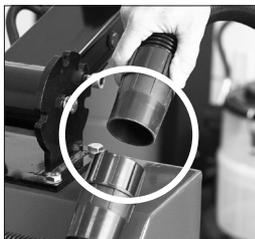
*connect the dust collector to the machine*
