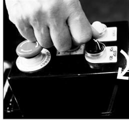
5. When starting the machine, the speed setting should be moderate: 6 or below. Use the Speed Control Switch to reduce or increase speed.
