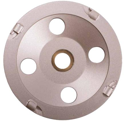
PCD (Polycrystalline Diamond) cup wheels are very different from segmented diamond cup wheels. Each segment is like a diamond tooth. These cups are specially designed for grinding off epoxy coatings, sticky mastic and heavy paint up to 5 times faster than standard diamond grinding cups.
