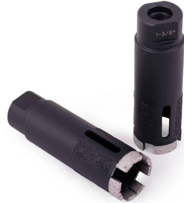
Our stone core bits are completely different from our tile bits. Premium diamonds and metals in the segments cut through the hardest stone easily. Brazed diamonds on the outside of the barrel keep the bit from binding in the hole. Brazed diamonds on the inside of the barrel allow the plug to fall out when finished coring. No more hammer and screwdriver to get the plug out.
