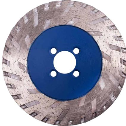
This unique blade is a combination granite diamond blade and grinding cup. The outer edge cuts even hard materials like granite and concrete. The underside is a premium grinding cup. It is perfect for simultaneously cutting off the old thin set while grinding the floor smooth.
