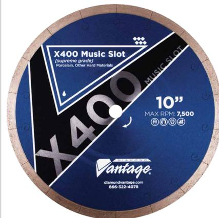
This supreme quality blade is designed to cleanly cut the hardest porcelain and ceramic tiles. Laser cut slots in the rim help to draw in air and water to keep the blade from overheating.
