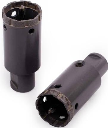
These bits have a bond designed to handle ceramic, porcelain and natural stone tiles. We offer them with either a 3/8" male stem for drills or a 5/8-11 female thread to fit any grinder or polisher. Available from 1/2" to 2".
