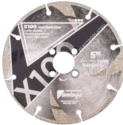
Next to glass, marble and travertine might be the most difficult material to cut clean. This blade has fine grit electroplated diamonds on both the edge and the face of the blade. It makes smooth chip free cuts in all calcium based natural stones like marble, limestone and onyx. Add our flush cutting adaptor and you can cut then sand the material.
