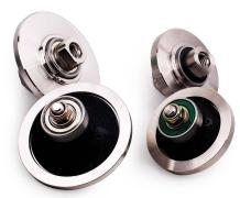
These bits have a 5/8-11 female thread to fit any grinder or polisher. Large brazed diamonds quickly shape porcelain, stone and concrete to demi bullnose, full bullnose or 45 degree bevel shapes. The stainless steel bearings keep the bit from going into the material too far in or down. So simple anyone can now make their own base board and finished trim tiles. Can be run wet or dry.
